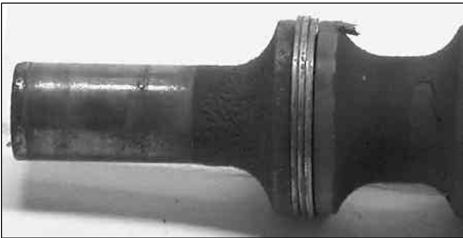
Above: The rear of the bolt before cleaning. The gas rings were almost stuck together and the carbon buildup was rock hard.
