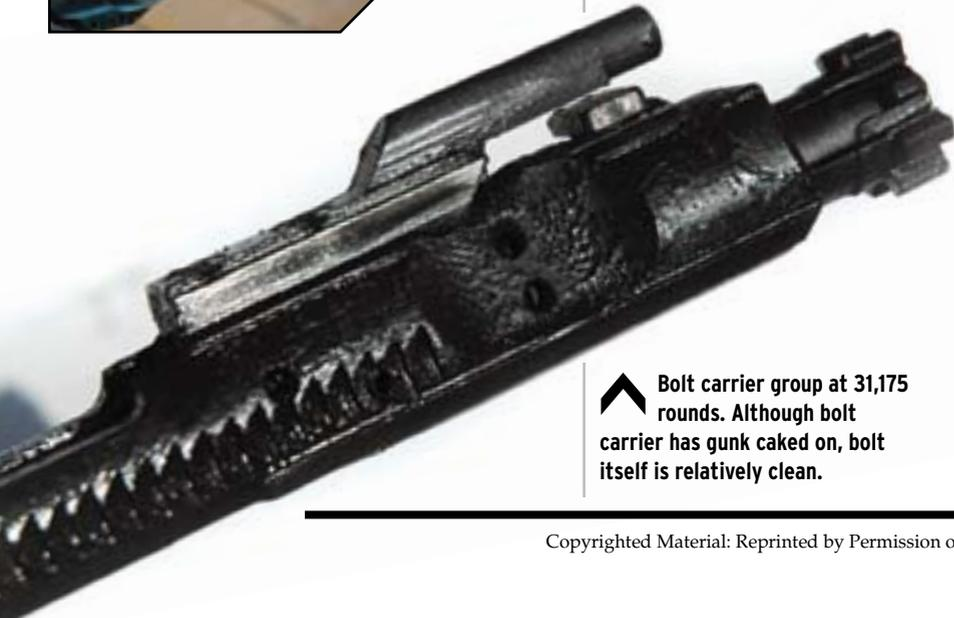
▲ Bolt carrier group at 31,175 rounds. Although bolt carrier has gunk caked on, bolt itself is relatively clean.
